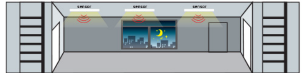
When insufficient light, the fixtures turn on at desired dimming level (10% - 50%).
